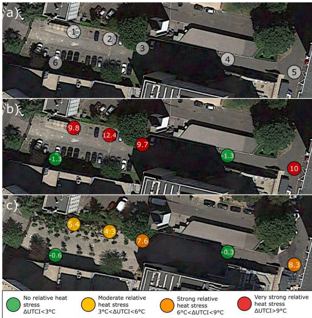
Fig. 13. a) Measurement points, b) thermal over-stress before renovation (June 2018), c) thermal over-stress after renovation (September 2021).
