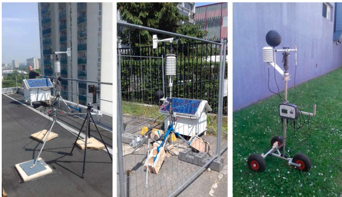
Fig. 4. Rooftop (left) and parking lot (center) fixed weather stations, and mobile (right) weather station (before conversion of the site).
